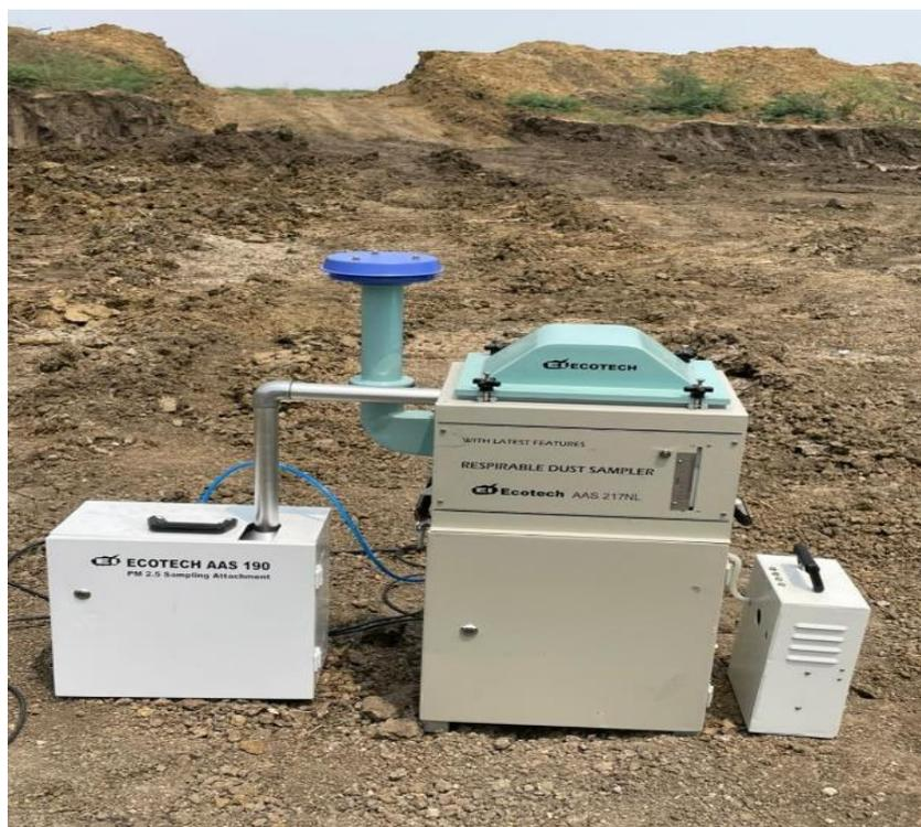
**Fig. 2: Respirable dust sampler (Ecotech AAS 190) (PM<sub>10</sub>) and Particulate dust sampler (Ecotech AAS127) (PM<sub>2.5</sub>)**
